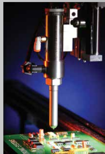
Nordson SC-300 Swirl Coat applying conformal coating.
